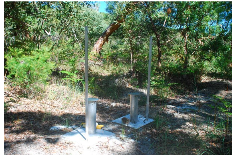
each pipe is to a different depth
